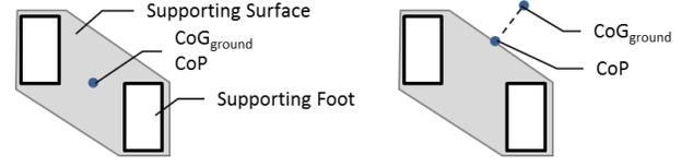
Fig. 3. The Center of Gravity projected on the ground and the Center of Pressure under (left) a balanced configuration, and (right) a potentially unbalanced configuration.
